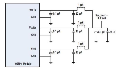
**Recommended Host Board Power Supply Circuit**
