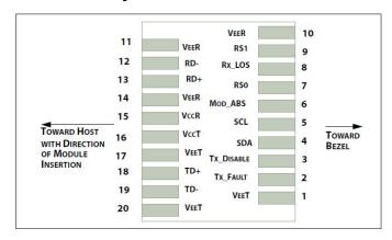
Host PCB SFP+ pad assignment top view
