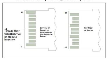
SFP+ module contact assignment
