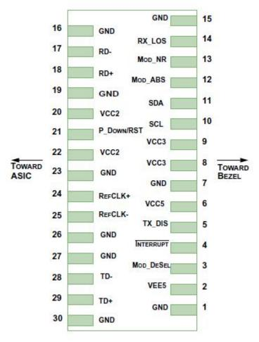
Host PCB XFP Pinout Top View
