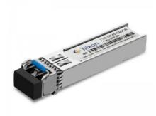
The SFP CWDM optical transceivers are high performance, cost effective modules. They offer the customer a range of design options, including optional DDMI, standard or extend temperature ranges. They are designed to provide Gigabit Ethernet compliant connections. These transceivers are qualified in accordance with GR-468-CORE.
