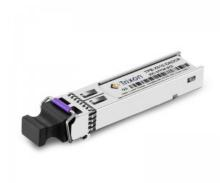
The TPB-X510-xxDCR is an 1330nm/1270nm DFB 25Gigabit SFP28 transceiver. It is designed to transmit and receive optical data over 9/125?m single-mode optical fiber (SMF) and support up to 10km. The module has a duplex LC optical interface and all mechanical characteristics are compliant with the current SFP28 specification (SFF-8431 and SFF-8432).
