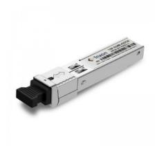
The GEPON OLT transceiver is small form factor pluggable module for serial optical data communications such as IEEE 802.3ah 1000BASE-PX20+. It is with the SFP 20-pin connector to allow hot plug capability. This module is designed for single mode fiber and operates at a nominal wavelength of 1490 nm. The transmitter section uses a 1490nm DFB laser and is a class 1 laser compliant according to International Safety Standard IEC-60825.
