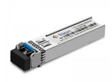
The GBE Bidirectional SFP optical transceivers are high performance, cost effective modules. They offer the customer a range of design options, including optional DDMI, standard or industrial temperature ranges. They are designed to provide Gigabit Ethernet compliant connections for 1.25 Gbps at short, intermediate and long reach links. These transceivers are qualified in accordance with GR-468-CORE.
