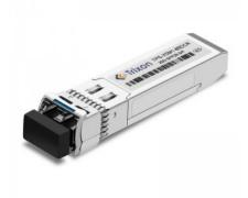
The TPS-X5M1-85DC(I)R is an 850 nm VCSEL 25Gigabit SFP28 transceiver. It is designed to transmit and receive optical data over 50/125?m multimode optical fiber (MMF) and support up to 70m on OM3 MMF and 100m on OM4 MMF. The module has a duplex LC optical interface and all mechanical characteristics are compliant with the current SFP+ specification (SFF-8431 and SFF-8432).
