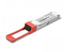
Trixon 40G 10km QSFP+ LR4 and ER4 Transcevier products is a 4x10G hot pluggable optical transceiver. The optical connectivity is based on two SMF LC connetors, one for Tx and one for Rx. The Tx and Rx each consist of 4 10GB/s CWDM channels, whose wavelengths are in the 1300nm range. The QSFP+-LR4 and ER4 transceiver is designed for applications based on the IEEE802.3ba 40GBASE-LR4 standard of up to 10km,40GBASE-ER4 standard of up to 40km reach.
