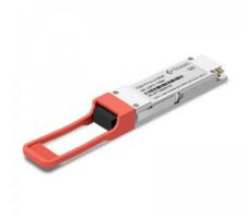
The TQS-FG10-31DCM is a parallel 40Gbps Quad Small Form-factor Pluggable (QSFP) optical module. It provides increased port density and total system cost savings. The QSFP+ full-duplex optical module offers 4 independent transmit and receive channels, each capable of 10.31255Gbps operation for an aggregate data rate of 40Gbps over 10 km.
