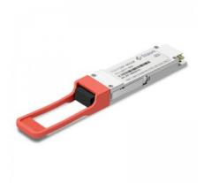
The TQS-FGM1-85DCR is a parallel 40Gbps Quad Small Form-factor Pluggable (QSFP) optical module. It provides increased port density and total system cost savings. The QSFP full-duplex optical module offers 4 independent transmit and receive channels, each capable of 10Gbps operation for an aggregate data rate of 40Gbps over 100 meters of OM3 multi-mode fiber. An optical fiber cable with an MPO/MTPTM connector can be plugged into the QSFP module receptacle.
