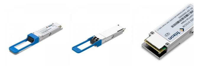
The TQS-HG02-31DCM is a parallel 100Gbps Quad Small Form-factor Pluggable (QSFP) optical module. It provides increased port density and total system cost savings. The QSFP28 full-duplex optical module offers 4 independent transmit and receive channels, each capable of 25.78125Gbps operation for an aggregate data rate of 100Gbps over 2000 meters.
