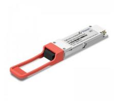
The TQR-HG10-31DCR-R is a parallel 100Gbps Quad Small Form-factor Pluggable (QSFP) optical module receiver. It provides increased port density and total system cost savings. The QSFP28 full-duplex optical module offers 8 independent receive channels, each capable of 28Gbps operation for an aggregate data rate of 100Gbps over 10km of single mode fiber.
