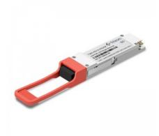
The TQR-HG10-31DCR is a parallel 100Gbps Quad Small Form-factor Pluggable (QSFP) optical module receiver. It provides increased port density and total system cost savings. The QSFP28 full-duplex optical module offers 4 independent receive channels, each capable of 28Gbps operation for an aggregate data rate of 100Gbps over 10km of single mode fiber.
