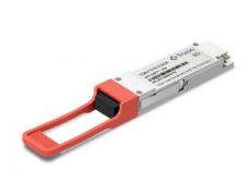
The TQS-HG10-31DCR is a parallel 100Gbps Quad Small Form-factor Pluggable (QSFP) optical module. It provides increased port density and total system cost savings. The QSFP28 full-duplex optical module offers 4 independent transmit and receive channels, each capable of 25.78125Gbps operation for an aggregate data rate of 100Gbps over 10km of single mode fiber.
