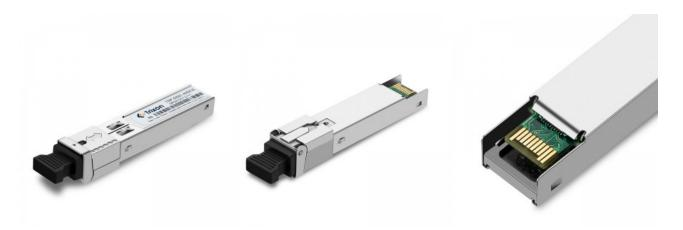
The GPON OLT transceiver is small form factor pluggable module for serial optical data communications such as ITU-T G.984. It is with the SFP 20-pin connector to allow hot plug capability. This module is designed for single mode fiber and operates at a nominal wavelength of 1490 nm. The transmitter section uses a 1490nm DFB laser and is a class 1 laser compliant according to International Safety Standard IEC-60825.
