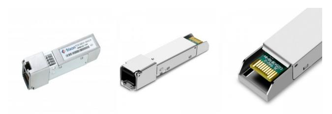
The 10/100/1000BASE-T Copper SFP Transceiver is small form factor pluggable transceiver. They are compatible with SFF-8074i Multi- Sourcing Agreement (MSA) and comply with Gigabit Ethernet standard as specified in IEEE Std 802.3. They are compliant with RoHS and lead-free per Directive 2002/95/EC. The physical layer IC (PHY) can be accessed via I2C bus, allowing access to all PHY settings and features.
