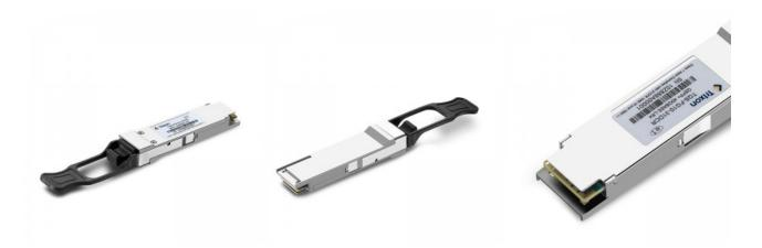
Trixon 40G 10km QSFP+ LR4 Transcevier products is a 4x10G hot pluggable optical transceiver. The optical connectivity is based on two SMF LC connetors, one for Tx and one for Rx. The Tx and Rx each consist of 4 10GB/s CWDM channels, whose wavelengths are in the 1300nm range. The QSFP+-LR4 transceiver is designed for applications based on the IEEE802.3ba 40GBASE-LR4 standard of up to 10km reach.
