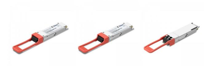
The TQS-HG30-31DCR is a parallel 100Gbps Quad Small Form-factor Pluggable (QSFP) optical module. It provides increased port density and total system cost savings. The QSFP28 full-duplex optical module offers 4 independent transmit and receive channels, each capable of 25.78125Gbps operation for an aggregate data rate of 100Gbps over 30km of single mode fiber.
