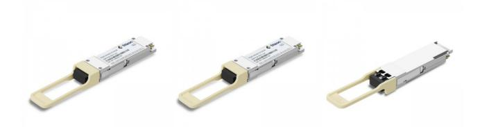
The TQS-HGM1-85DCR is a parallel 100Gbps Quad Small Form-factor Pluggable (QSFP) optical module. It provides increased port density and total system cost savings. The QSFP28 full-duplex optical module offers 4 independent transmit and receive channels, each capable of 25.78125Gbps operation for an aggregate data rate of 100Gbps over 100 meters of OM4 multi-mode fiber.
