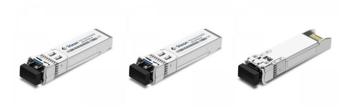
The TPS-X510-31DCR is an 1310nm DFB 25Gigabit SFP28 transceiver. It is designed to transmit and receive optical data over 9/125?m single-mode optical fiber (SMF) and support up to 10km. The module has a duplex LC optical interface and all mechanical characteristics are compliant with the current SFP+ specification (SFF-8431 and SFF-8432).
